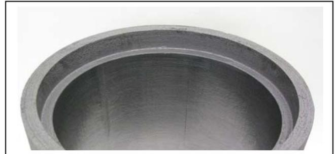
**CONSTRUCTION:** RFC is produced by laminating multiple layers of soft felt with a resin and firing it to 1,900°C. As an option, graphite foil may be bonded to any surface specified to lower the emissivity and minimize process gas infiltration. Graphite Paint can also be coated on select surfaces to reduce particle generation.
